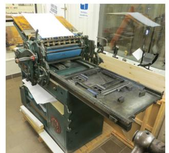
At the far end of the room is a galley press. It has been used ▶ primarily for making impressions for proofreading and for sending proofread texts to clients for approval. It is the only cylinder press at the museum. All the other presses are platen presses, whereby a flat metal plate presses the paper against the colored surface (the forme).
