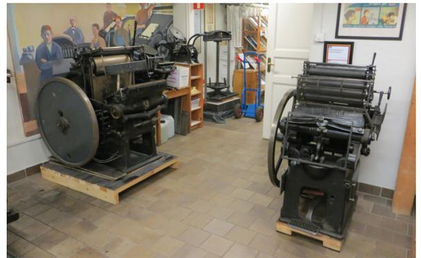
◀ The Heidelberg Press, commonly called “the Wing”, is most likely the best-selling press in the world. The basic construction was finished as early as 1914, but continuous improvements were made later. The press was manufactured in Germany until 1985 and then for a while in Czechoslovakia. It is still in use at many printing houses around the world. This press is our only automatic press, where the paper is fed in and out automatically.
