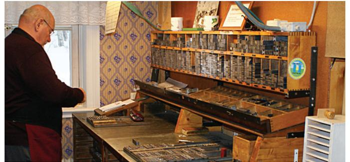
▲ The work benches are of the “newer” model, with flat work surfaces. In the early 1920s they replaced the tilted work benches (on display in our exhibition hall) for hand composing longer texts (ox setting) was replaced by machine compositors. The benches are called shelves and contain a number of drawers for storing different fonts.
